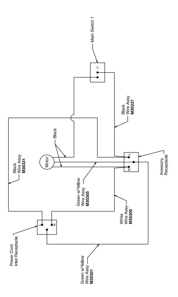
Wiring Diagram 100/120V
